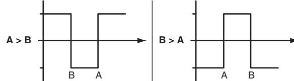
Teach in switching thresholds: you can teach in or overwrite a taught-in switching threshold at any time. To do this, press the "TI" button again.
